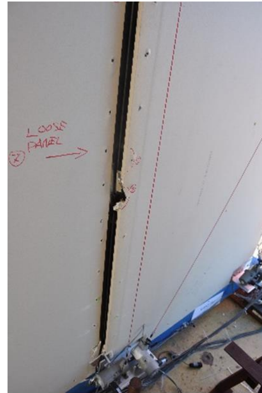
Extensive damage to Gypsum boards
