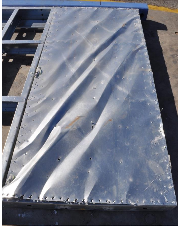
Shear buckling of steel sheet
