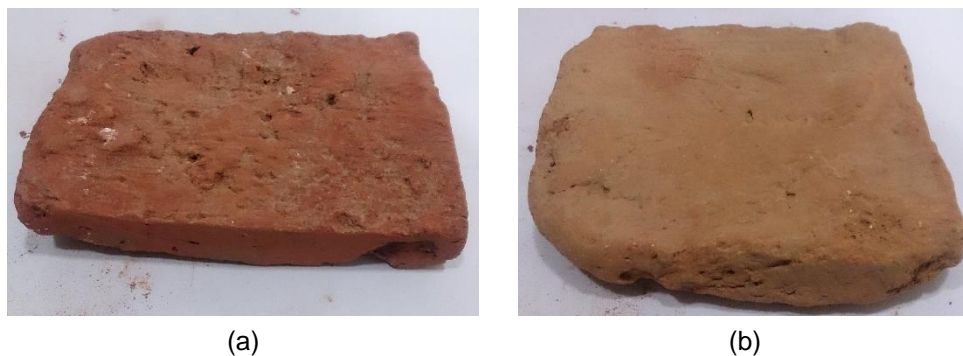
Figure 4.5. Lakhaury bricks: (a) Fully baked brick and (b) Partially baked brick
